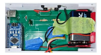
It is a pretty simple build, here is whats inside: There are only 7 electronic components plus battery, battery holder, BNC connector and switch. Time to build about 30 minutes.
