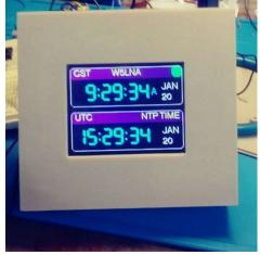
It shows both local and UTP time. It has battery backup and automatically adjusts for Daylight Savings Time. It has a battery charger board and will run for a good 3-4 hours on battery. It has a 2.8" TFT display, It's a fairly simple project to build and it will introduce you to programming an Arduino. (Actually, it will introduce you to loading a program written by others but configured by you.)
