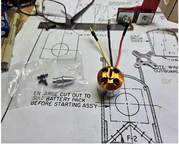
Here is a picture of the motor. Notice it has 3 wires. This is a brushless motor that puts out about 200 watts of power and is about 70%-85% efficient. They're are quite interesting as they are essentially an AC motor that runs off a DC battery but require a motor controller to make them work. If weather permits, Ill try and add a video of it flying....weather permitting.
