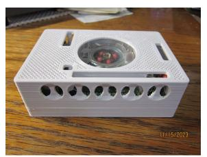
Here is the 3D printed case for the PI once the project is complete. Notice the cooling fan. It is a must for the PI 4 and the P5. They run a bit warm without one.
