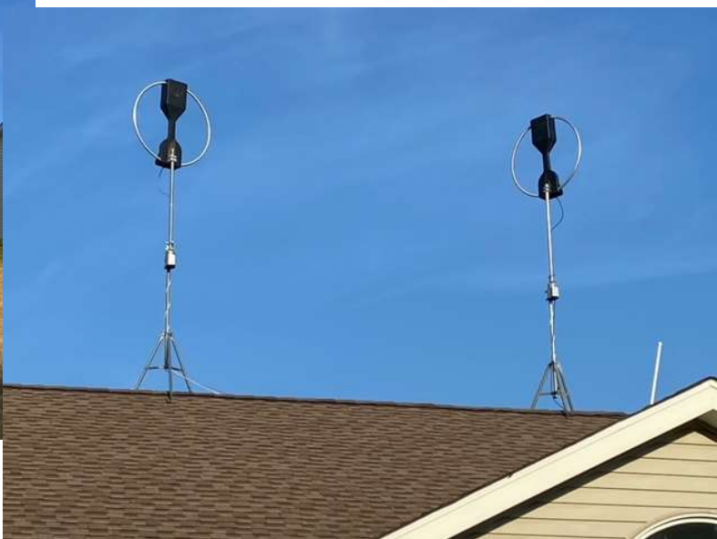
My antennas: The left one is 10-30 Meters the Right is 20-49 meters
