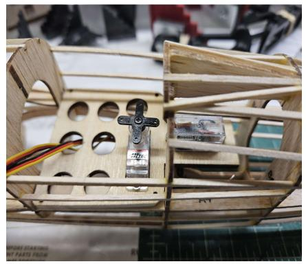
Close up photo of the cockpit area with the 2 servos installed. For perspective, the cockpit area is about 2.5" wide x 2.5" long. These servos will operate the rudder and elevator using Upholstery thread in a Pull\Pull configuration.
