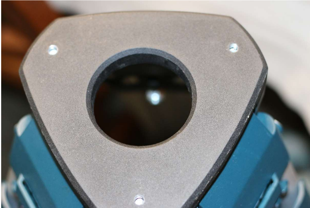
Top of tripod with holes drilled and tapped
