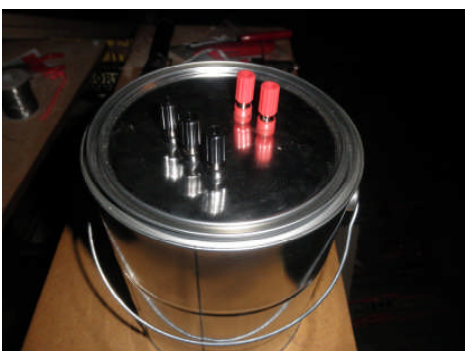
This allows the load to be configured for 50 Ω, 100 Ω, 200 Ω, 300 Ω, 400 Ω, 600Ω and 800 Ω.
